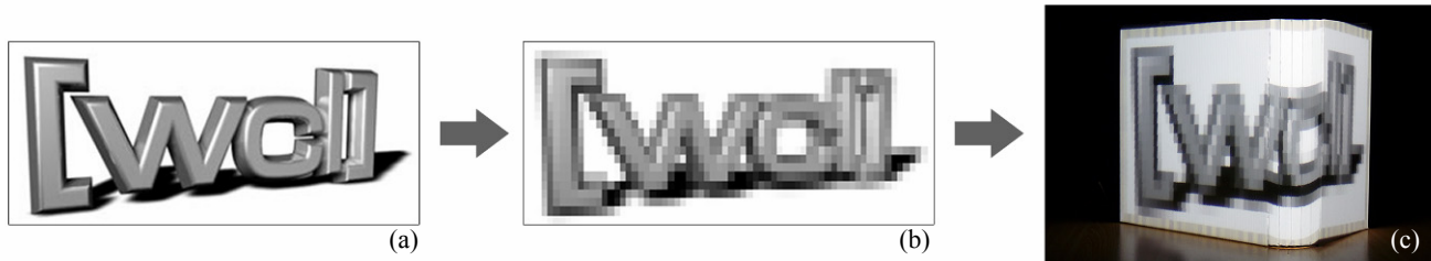
Figure 2. Stages of the simulation. Original logo in a picture viewer program (a), scaled down to the resolution of the Lantern (b), and applied to a model of the Lantern through the use of SAR (c). The scaled texture is also used in the simulation application.
