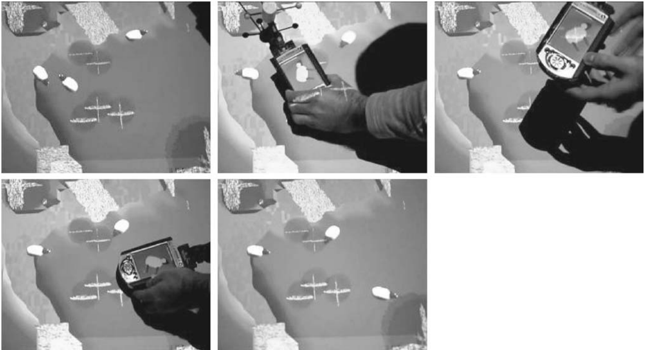
Fig. 10 Scooping a virtual sheep with an iPAQ that acts as tangible display
