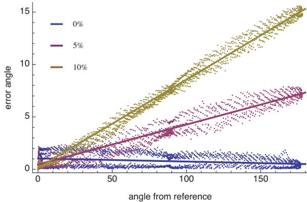
Figure 3: Correlation between the error of the visual tracker and the angle to the reference frame.
